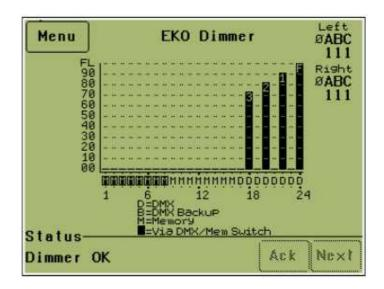
In the example above channels 1 to 8 are switched via the DMX/Mem switch, which is currently switched to Memory source. Channels 9 to 17 are sourced from Memory. Channels 18 to 24 are sourced from DMX, which is connected.
